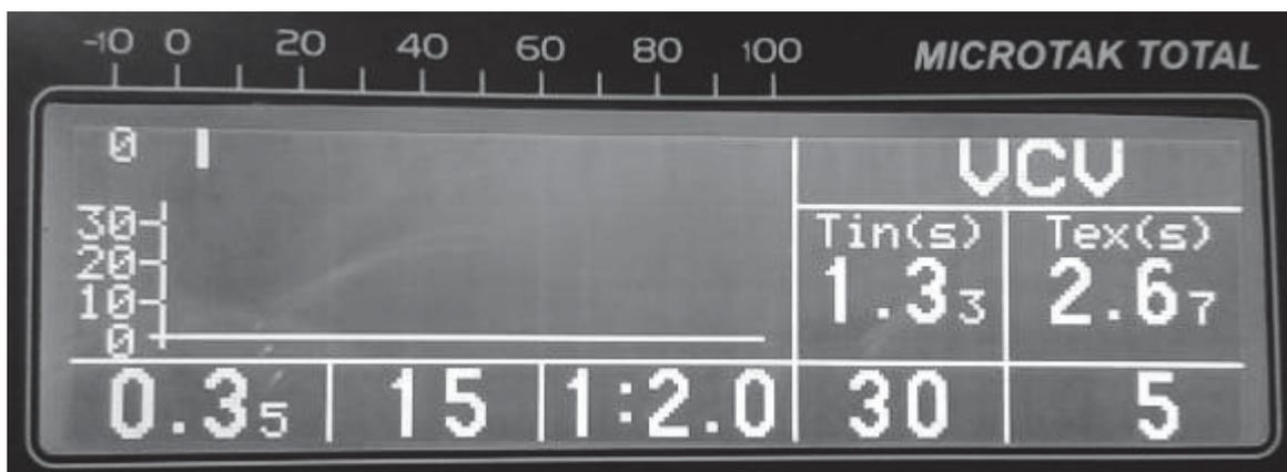
**Figura 7.3: Tela principal do Ventilador MICROTAK TOTAL.**
